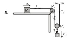
Relative between  $a_1 \& a_2$   $a_1 = 2a_2 = 2a$ Relative between  $T_1 \& T_2$   $T_2 = 2T_1 = 2T$   $T_1 = M_1a_1$  .....(i)  $M_2g - T_2 = M_2a_2$  .....(ii)  $2T = 4M_1a$  $M_2g - 2T = M_2a$
